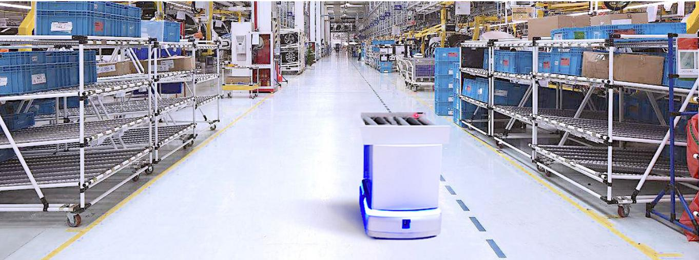
**Moving Robot** leverages advanced SLAM laser navigation method to identify factory's environment and schedule the route independently. The robots are able to avoid the obstacle to deliver pallet / rack to the destination in a flexible and smooth way.
